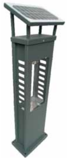
Material :Aluminum Solar panel: 5W LED: 3W ( Epistar) Battery:6V/4.5AH Height:75cm
