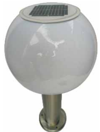
Lamp house dia. 250mm Solar panel: 1W LED: 0.5W(Epistar) Battery:3.6V / 2300mAh Height: 60cm
