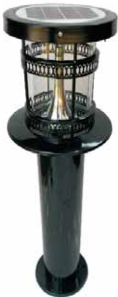
Material :Aluminum Solar panel: 3W LED: 2W( Epistar) Battery:6V/4.5AH Height: 80cm
