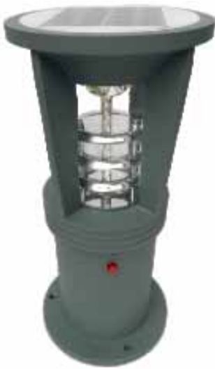
Material :Aluminum Solar panel: 3W LED: 2W (Epistar) Battery:6V/4.5AH Height:45cm
